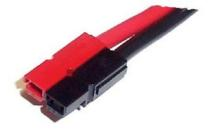
The plastic housings are held together with dovetail joints. Always slide these joints together! They will be damaged if you try to snap them together or apart. They ONLY slide together in one direction. This should be obvious by looking at them carefully.
